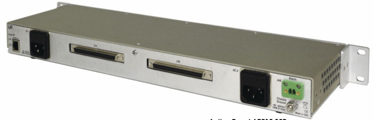
Active Panel AP512-32B 1RU unit shows expansion ports (for 1024x1024), dual AC inputs, 1Gb Ethernet port, ground stud and hard contact alarm port
